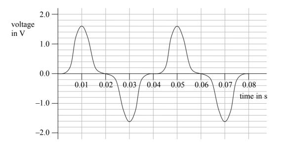
The maximum output voltage of this dynamo is about
