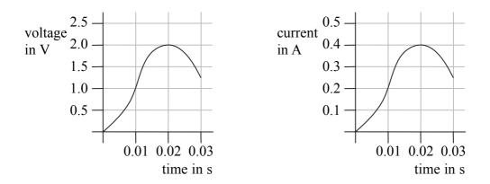
When the time is 0.02 s the output **power** of this dynamo is
