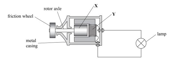
25. Which row of the table is correct for X and Y in the dynamo?
