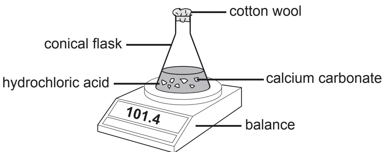
The student measured the mass of the flask and its contents for 8 minutes.
