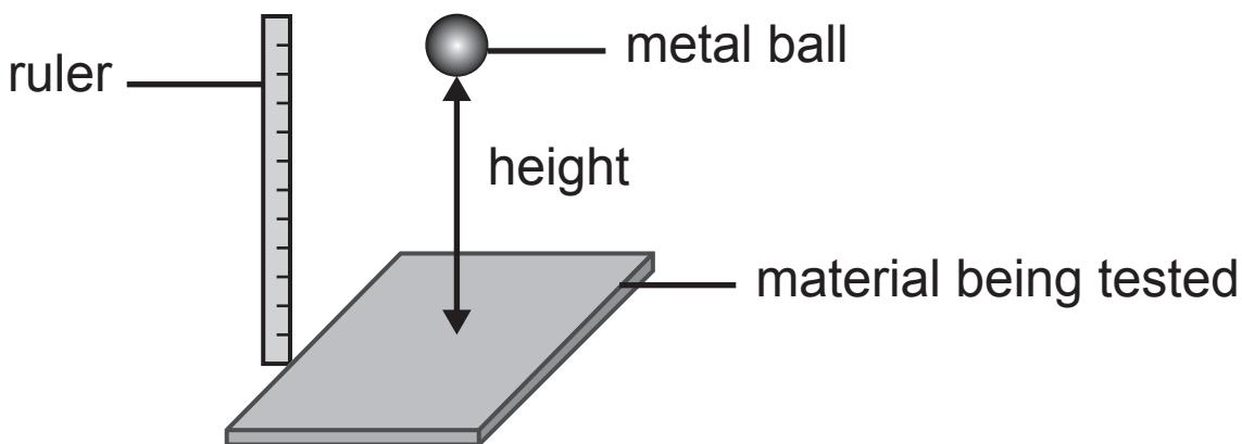
The height the ball was dropped from was increased until the material cracked when hit.
