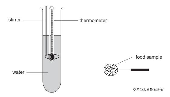
Describe how you would compare the amount of energy released from a biscuit to the amount of energy released from bread, using the apparatus above.
