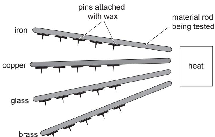
The number of pins still attached to each rod was recorded after 1, 3 and 5 minutes. The results are shown in the table below.
