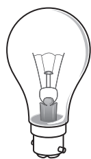
filament lamp (wire inside)
