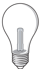
halogen lamp (filled with argon)
