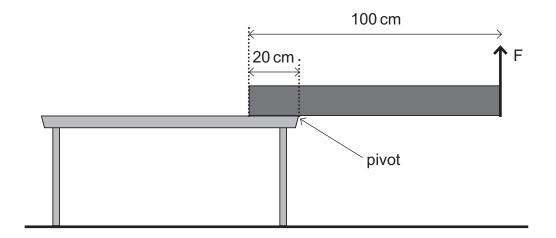
Calculate the upward force, F.
