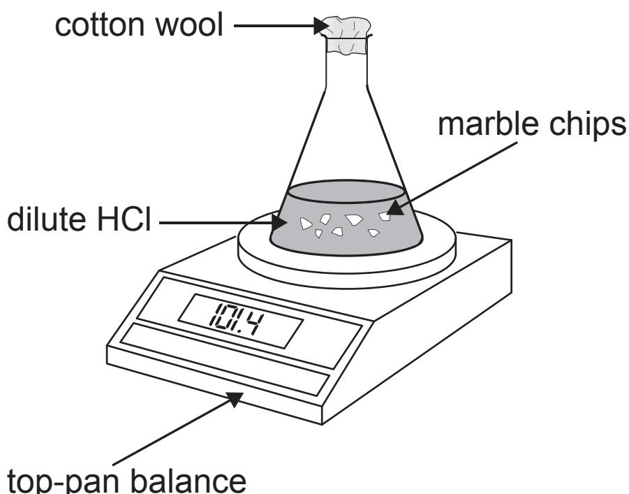
The student measured the mass of the flask and its contents every minute for 8 minutes.
