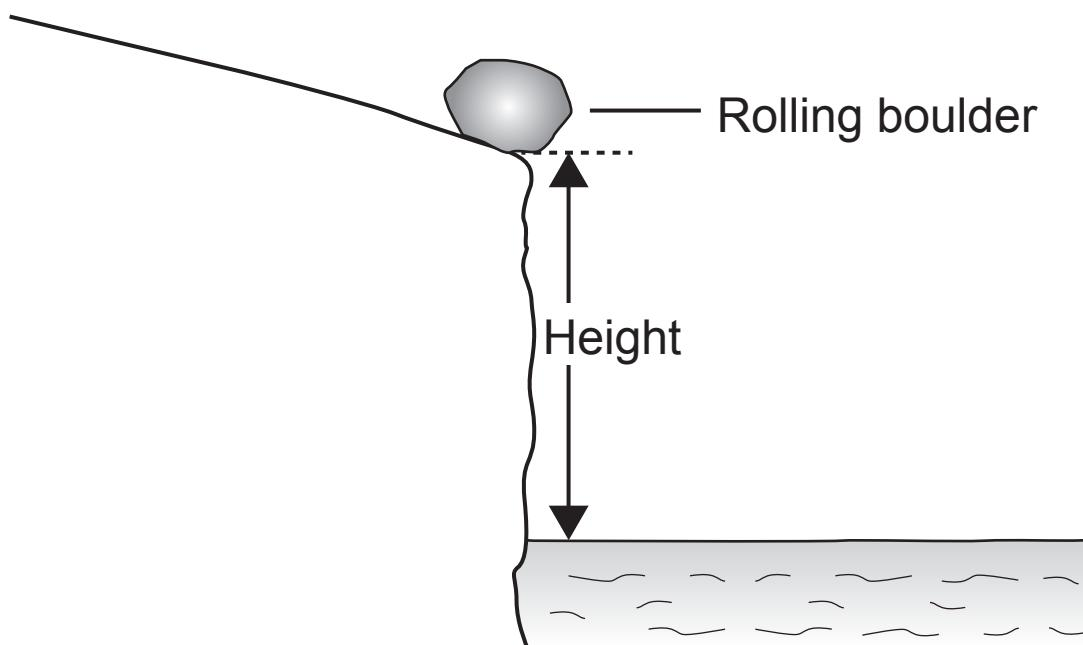
In the position shown at the edge of the cliff the boulder has a kinetic energy of 3520 J and a potential energy of 52 800 J.
