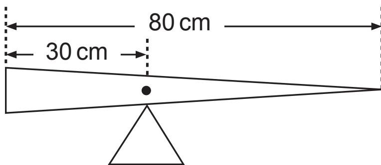
We now know that the position of the centre of gravity of the plank is 30 cm from the left-hand end and this is indicated by a dot as shown.
