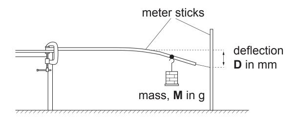
According to theory, the mathematical relationship between the deflection (D) of the beam and the mass (M) hung from the beam is given by
