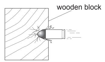
The average resistive force acting on the bullet as it becomes embedded in the wood is 1960 N. The bullet stops a distance of 15.0 cm into the wood.
