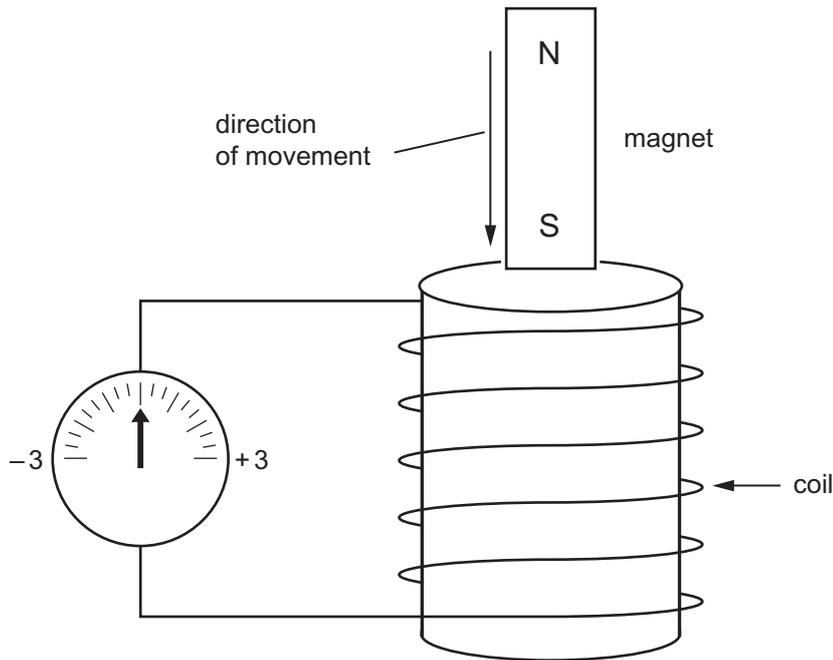
(a) When a pupil moves the magnet into the coil the needle on the ammeter moves to +2 and then returns to zero.
