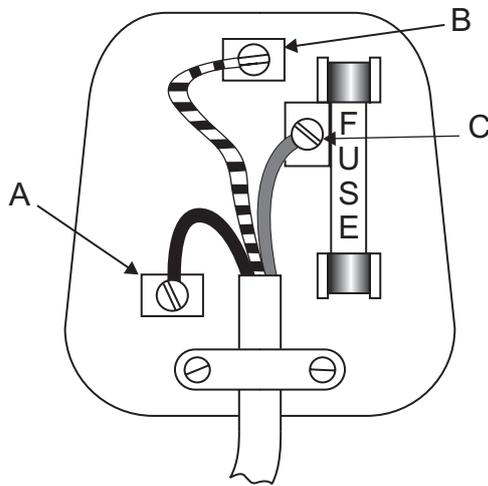
(i) Which pin A, B or C is the earth pin?
