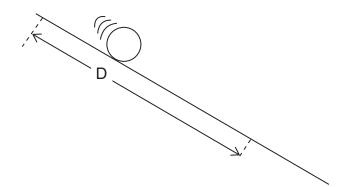
The time taken for the ball to travel a distance D was measured on three occasions and the average time T was recorded. This was then repeated for different distances.
