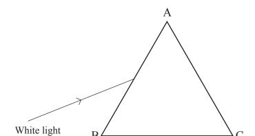
A prism may be used to split white light into its component colours.
