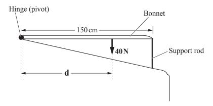
The support rod exerts an upward force of 24 N and the bonnet has a weight of 40 N. Calculate the distance **d** of the centre of gravity of the bonnet from the hinge.
