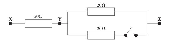
Complete the following table to show the total resistance between the different points for the switch settings indicated.
