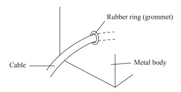
With use this grommet can wear away and the edge of the metal body can cut through the insulation in the electric cable.
