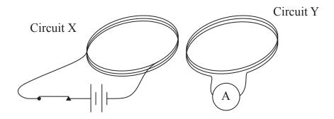
(ii) State three practical ways that a current can be induced in Circuit Y.
