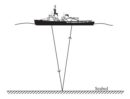
Calculate the distance between the ship and the seabed.
