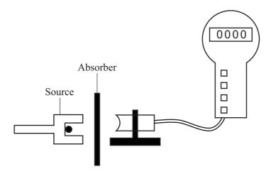
Two different types of absorber are placed one at a time between the detector and the source. For each absorber, a count is taken over ten minutes and the average number of counts per second worked out. The results are shown in the table.
