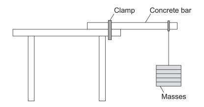
The engineer added masses to the concrete bar and recorded the mass needed to break the bar. She repeated each experiment once.
