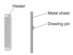
The student stuck the drawing pin onto the metal sheet using wax.
