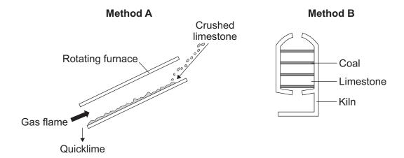
Method  $\bf A$  is a modern method. The crushed limestone is fed continuously into a rotating furnace by machinery. Quicklime falls out at the bottom and is removed by machine.
