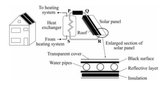
7A The different layers of the solar panel make the panel transfer solar energy in the most effective way.
