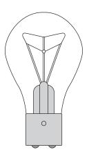
The lamp has a power of 100 watts (W). It gives out light at a rate of 5 watts.
