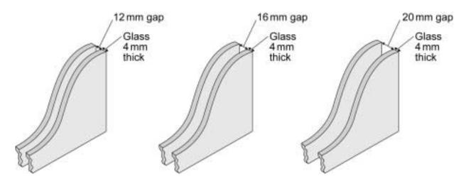
The gap between the two sheets of glass can be filled with either air or a mixture of air and argon.
