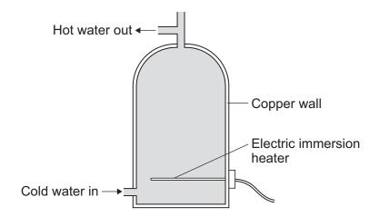
**5 (a)** Energy is transferred by the process of convection from the hot water at the bottom of the tank to the cooler water at the top.
