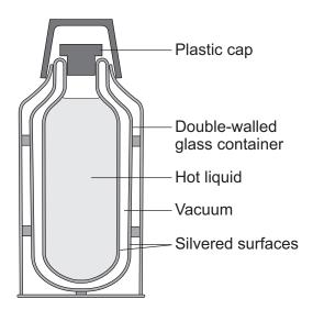
A vacuum flask is designed to reduce the rate of energy transfer by heating processes.
