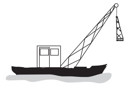
The girder has a weight of  $1\,000\,000\,\mathrm{N}$  and is lifted to a height of  $1500\,\mathrm{cm}$ .
