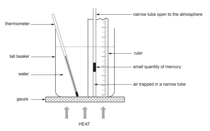
(a) In a class experiment the volume of a mass of air changed when it was heated. The air is shown contained in a narrow tube which is open to the atmosphere. The length of trapped air in the tube (which indicates its volume) was measured as the temperature of the water was changed. The results are shown in the table below.
