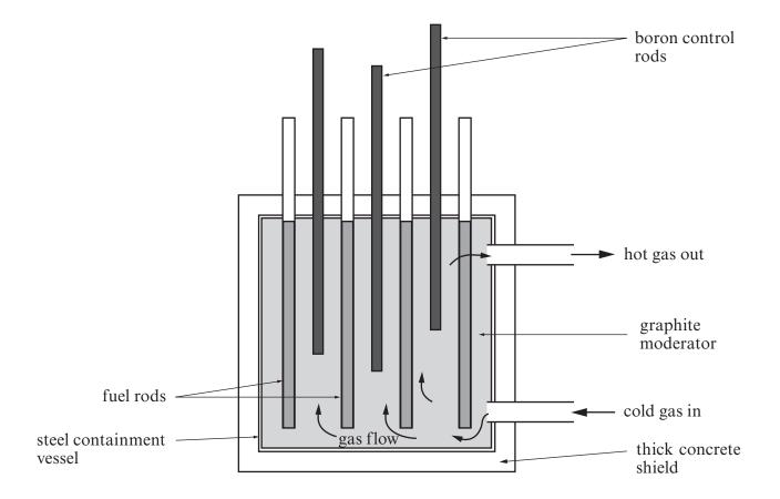
The fuel rods used in the core of a gas-cooled reactor are made of U-238 (Uranium-238) enriched with 3% of U-235 (Uranium-235). Only U-235 undergoes fission. Its atoms capture slow moving neutrons and split to produce two new radioactive nuclei and up to three new fast moving neutrons.
