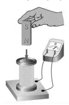
When the North Pole of the magnet is pushed into the coil, the meter needle flicks to the right and returns to the middle.
