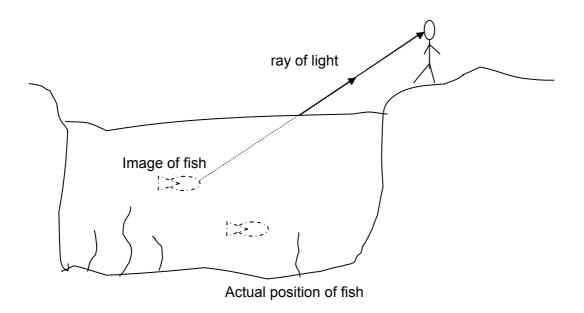
In actual fact the fish is not in that position but appears to be there due to the refraction of light as it passes from the water into the air.
