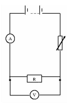
She adjusts the variable resistor and records five sets of values for voltage and current.
