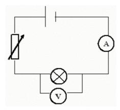
The pd (voltage) across the bulb is 12V when the current is 2A.
