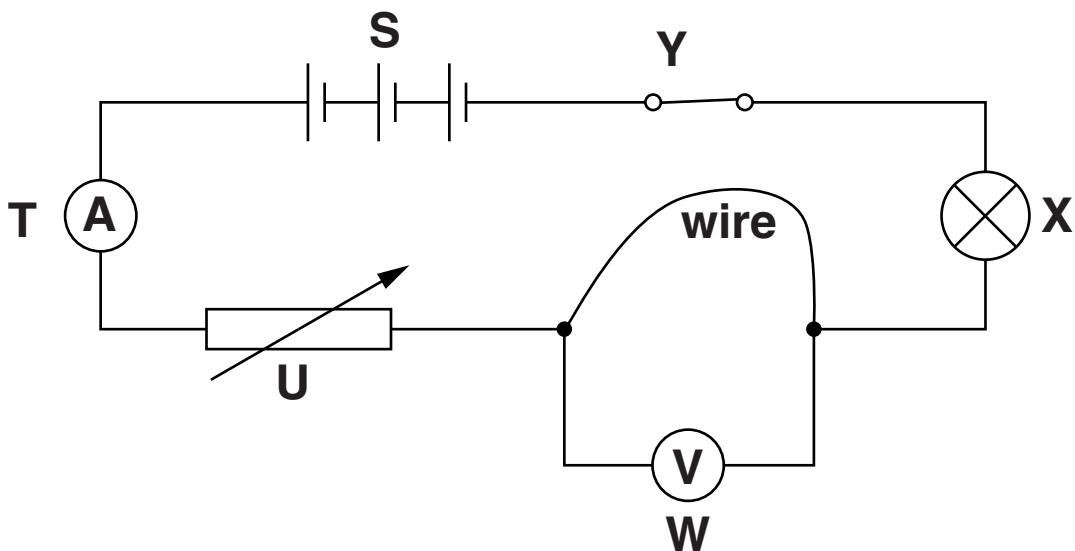
(a) There is a variable resistor (U) in the circuit.
