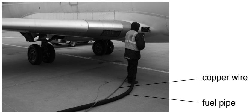
There is a copper wire between the aircraft and the fuel tanker.
