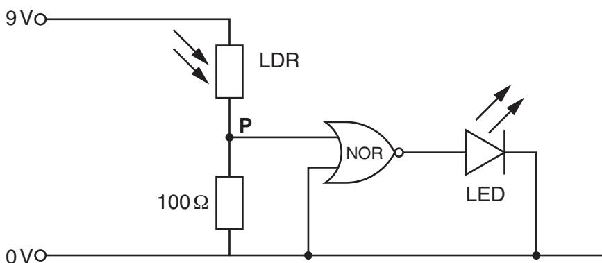
In the light, the resistance of the LDR is  $100\Omega$ .
