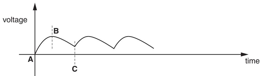
The capacitor smoothes the voltage output.
