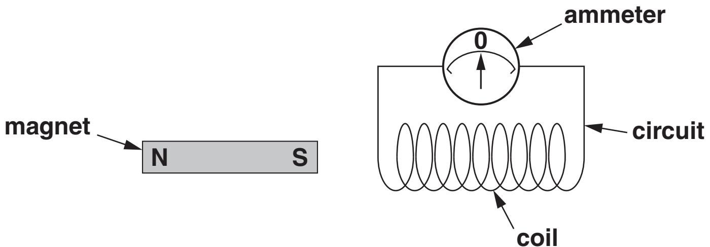
Emily moves the magnet towards the coil. A current flows in the circuit.
