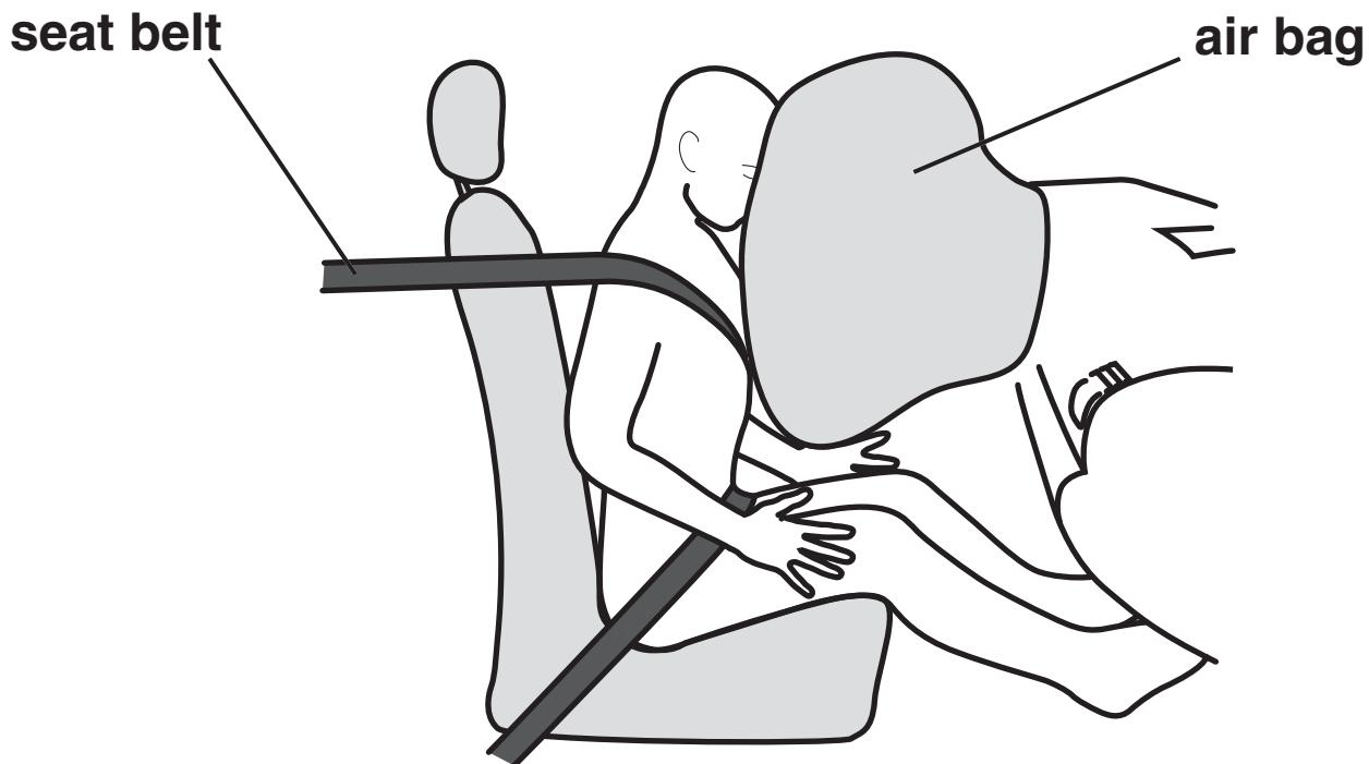
**The airbag and seatbelt change shape and absorb energy in the crash.**
