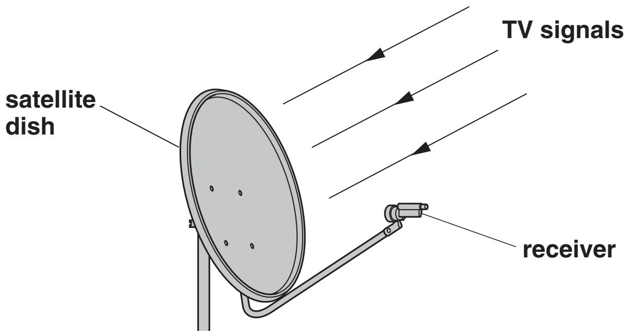
**The TV signals reach the satellite dish. They are then focused on the receiver.**
