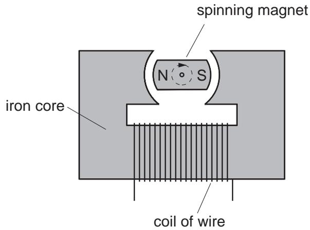
(a) Here are some voltage-time graphs for the voltage across the coil of wire as the magnet spins round.
