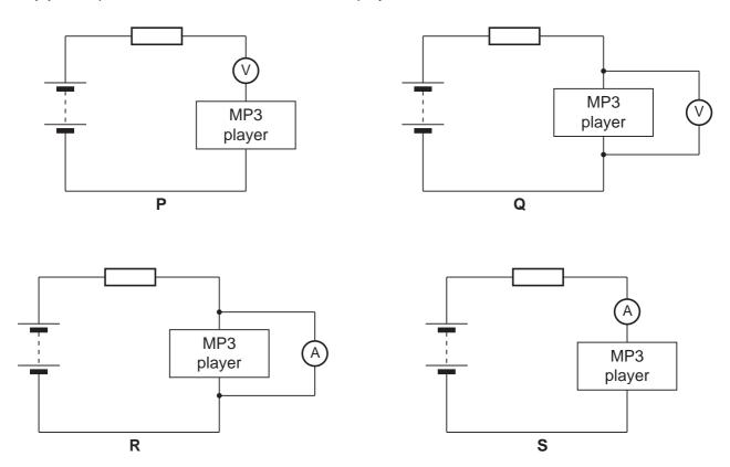
Which diagram, **P**, **Q**, **R** or **S**, shows how a meter should be connected to measure the potential difference across the MP3 player?
