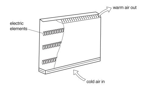
(a) The storage heater contains a box measuring 1.0 m long, 0.5 m high and 0.2 m deep.
