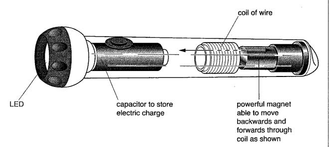
(a) Use your ideas about electromagnetism to explain how shaking the torch produces a current.
