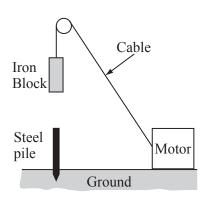
The motor does 30 kJ of useful work in raising the iron block above the steel pile. The electrical energy required to do this is 40 kJ.
