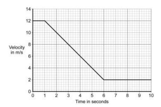
7 (a) Use the graph to calculate the distance the car travels while it is slowing down.
