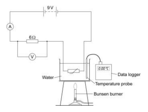
To calibrate the thermistor to measure temperature, the student placed the thermistor in a beaker of water at 0 °C and took the voltmeter reading. The student then heated the water slowly with a Bunsen burner. The student recorded the reading on the voltmeter every 10 °C.
