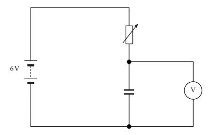
7.1 Which graph line, A, B, C or D, shows how the potential difference (voltage) across the capacitor changes as it is being charged?
