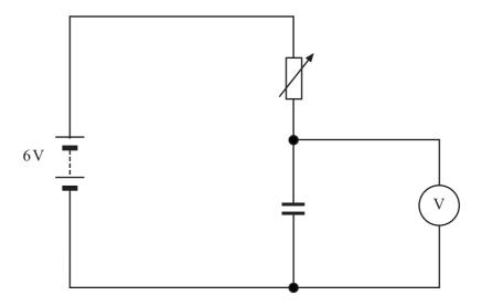
**10.1** Which graph line, **A**, **B**, **C** or **D**, shows how the potential difference (voltage) across the capacitor changes as it is being charged?
