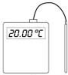
Temperature probe and data logger
