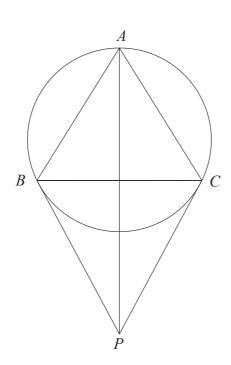
A, B and C are three points on the circumference of a circle. Angle ABC = Angle ACB. PB and PC are tangents to the circle from the point P.
