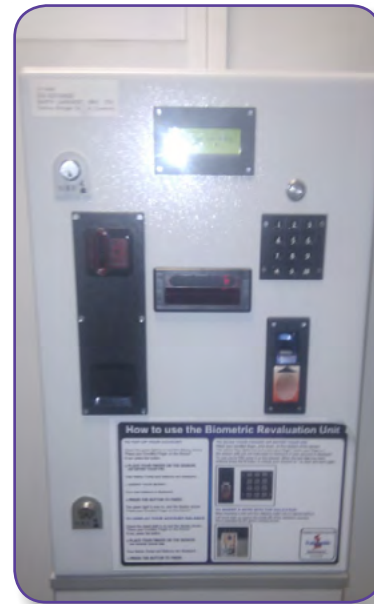
Figure 3. Payment machine that can be used by students to top up their account balance. The finger is scanned to retrieve the account details, then money is entered into the machine and the balance is updated. It happens in real time so the money can be used straight away
