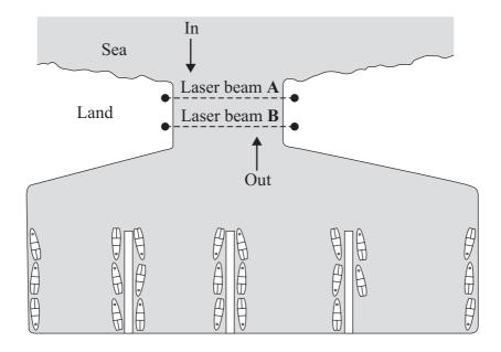
The computer uses two laser beams across the harbour mouth to tell whether a boat is entering or leaving. The computer can sense when a laser beam is broken.
