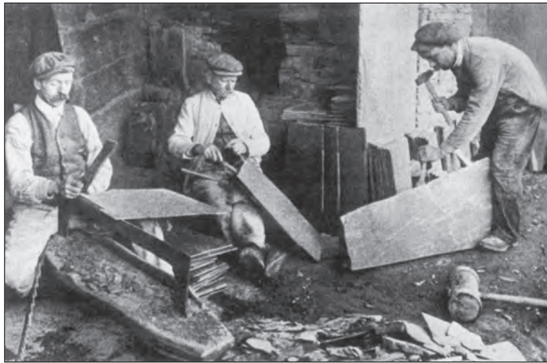
[Slate workers in North Wales preparing roofing slates in the early twentieth century]
