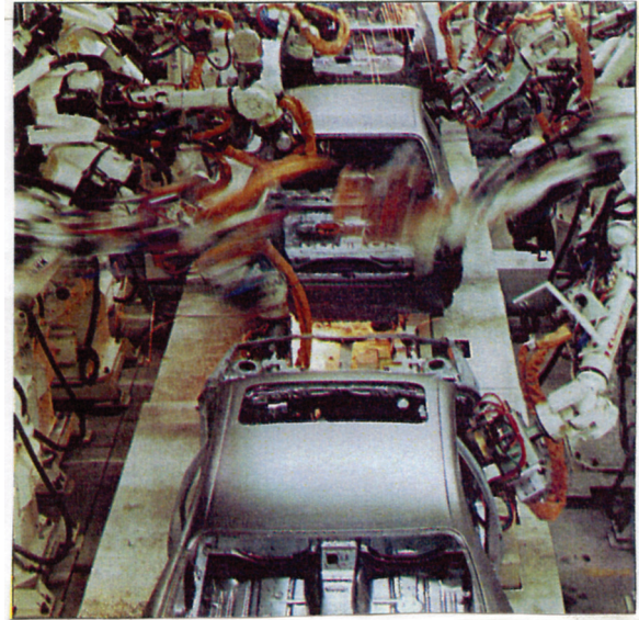
2 Robots weld the body shape together.
