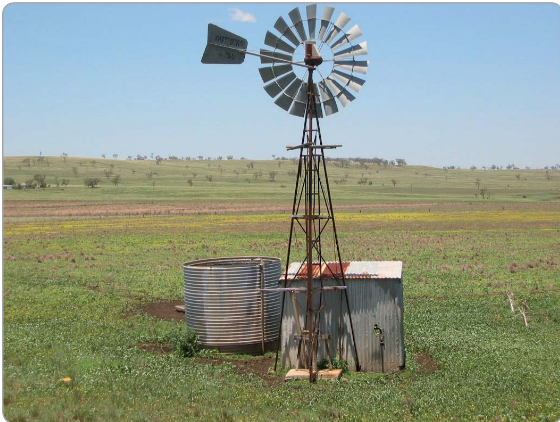
Figure 13 A wind pump used for pumping up groundwater
