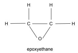
The raw material used to make epoxyethane is ethene. This is obtained by the cracking of hydrocarbons from petroleum.
