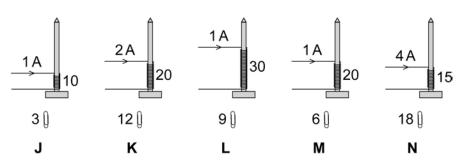
The student wants to find out how the strength of an electromagnet depends on the number of turns of wire in the coil.
