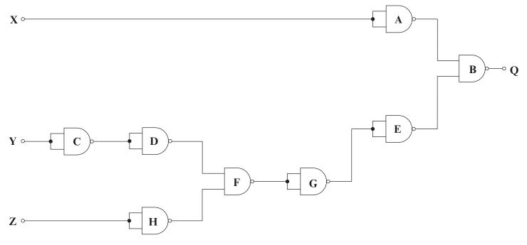
Which 2 pairs of gates are redundant? Circle the correct pairs.
