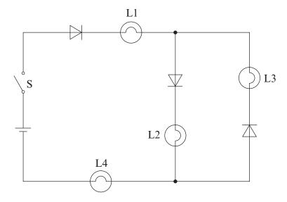
The Switch S is now closed. Which lamp, L1, L2, L3 or L4, will NOT light up?
